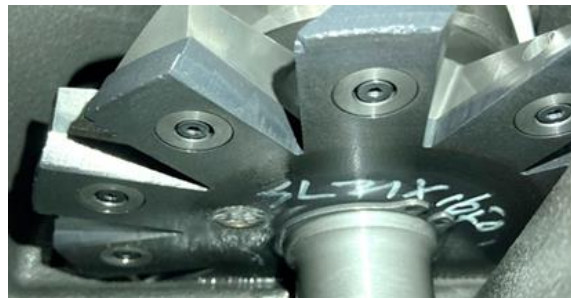
Figure 8: External View of bolt fixing of gate rotor
